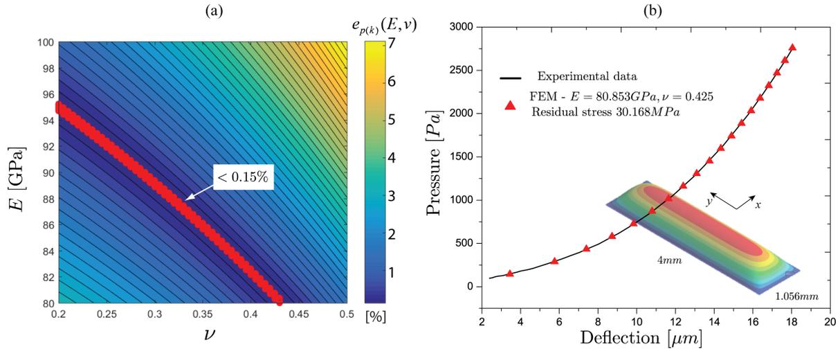
Figure 3. a)  $e_p(E, \nu)$  error function. b) Experimental and numerical load-deflection curves (Elastic thin film).
