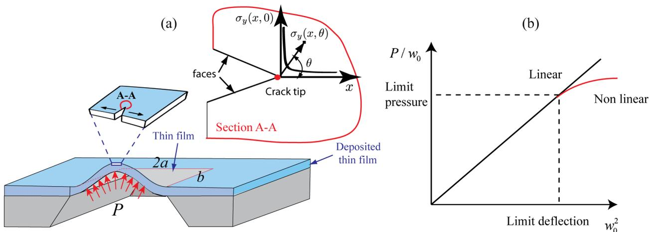
**Figure 1.** a) Bulge test on a cracked thin film (half model). b) Linear relation to establish limit points with the load-deflection parameters.
