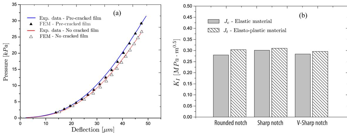
Figure 4. a) Comparisons in load-deflection curves for a non-cracked and cracked film with the experimental data. b)  $K_{IC}$  values obtained from different notches from J-integral.
