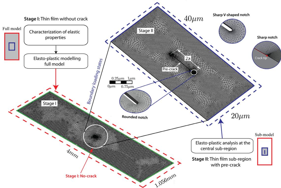
**Figure 2.** Scheme of the solution process by finite element analysis
