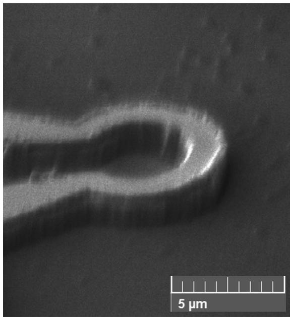
Side view at the antenna after RIE Etching
