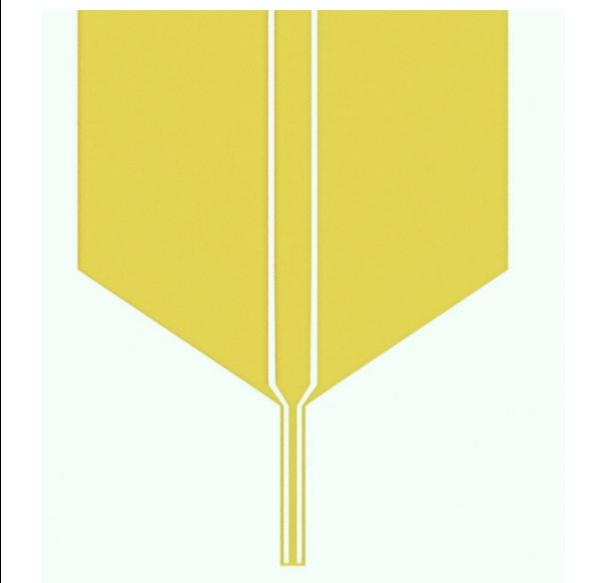
Coplanar waveguide type antenna
