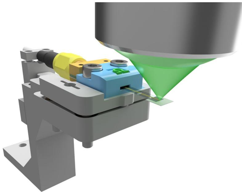
*Levitating antenna device with excitation part fabricated on a glass cantilever landed on a sample with magnetic nanostructures. Example of Brillouin light scattering experiment.*
