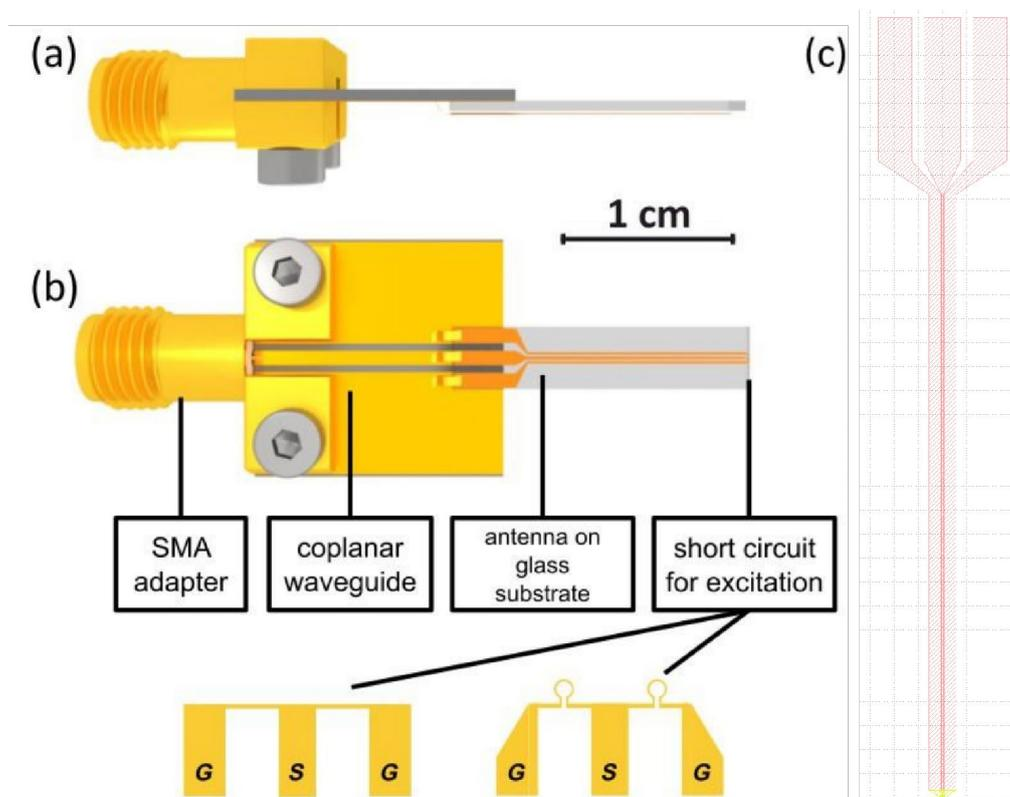
*Panel (a) side view and panel (b) top view of the completed antenna with designation of its components. Reprinted from [Hache20]. (c) GDS design of the antenna for EBL.*
