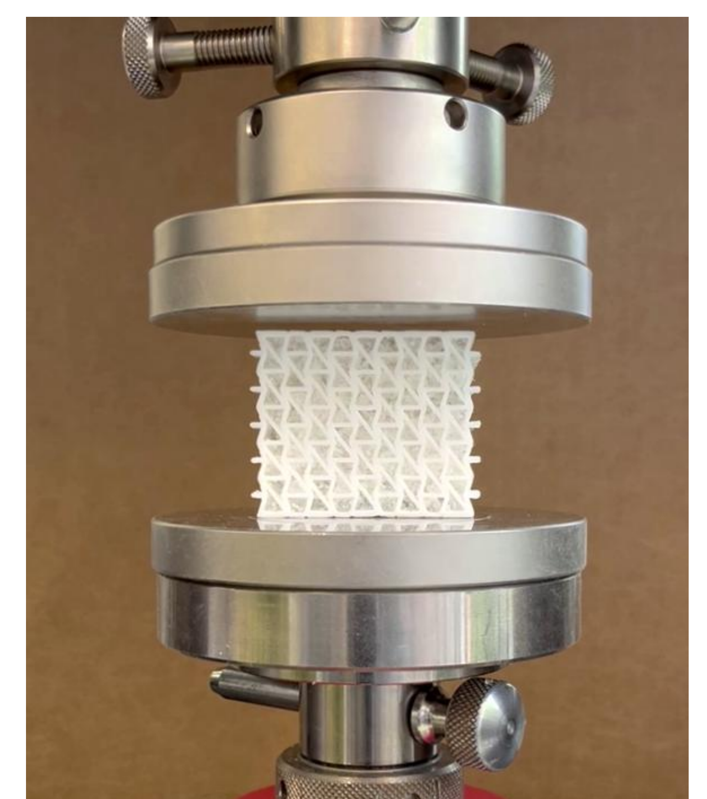
Figure 6: Compression test setup
