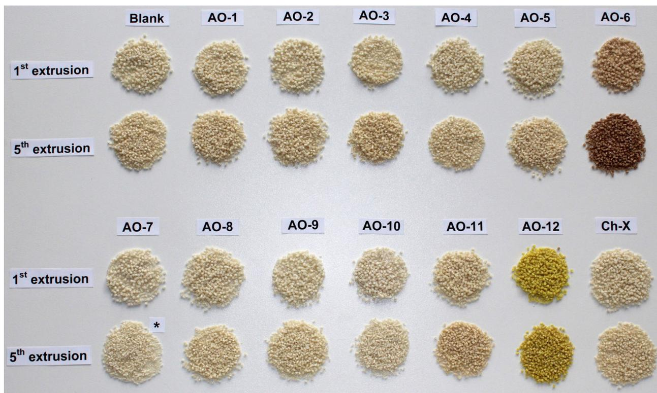
**FIGURE 10** Color development due to multiple extrusion at 190°C/60 rpm (\* = fourth extrusion) [Color figure can be viewed at [wileyonlinelibrary.com](http://wileyonlinelibrary.com)]
